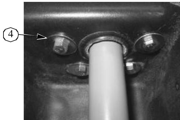
Figure 3. Inlet Pipe Support Installation
