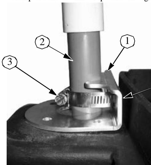
Slots in Inlet Pipe Support Bracket
