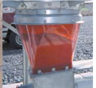
Red translucent boot transition offers highest durability and even flow
