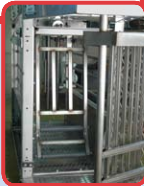
Trainer Gate in extended position.
