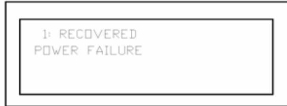
1) After power is reapplied to the controller, the above screen will appear.
