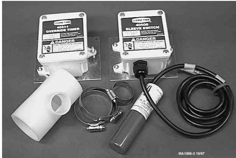
The 40508 Proximity Sleeve Switch is for use on the Multiflo™ Circulating Feeding Systems. The switch serves as the control to allow system operation and shut-off without unnecessary recirculation.
