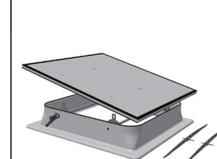
Once pins are removed, lift off lid and place in safe location.
