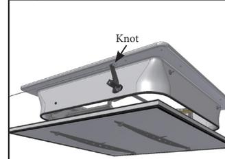
Attach string to Weight Arm with a regular knot. String should always be pulled parallel with inlet when inlet is being pulled shut.
