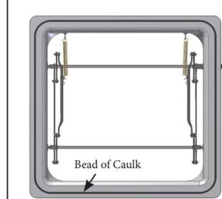
Place a bead of caulk around top side of inlet. Using 2" wood screws with a washer fasten inlet to ceiling. 8 screws placed 3/4" from outside edge.
