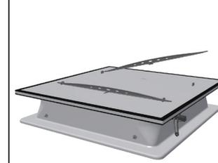
Remove Lid Pins by lifting on center pin until tab comes out of hole on lid. Then pull the pin sideways so that it bends enough to be freed.
