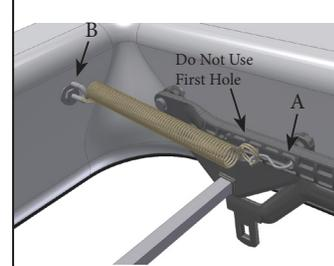
Hang S-hook into pre-drilled hole (A). Attach spring on S-Hook and J-Hook (B). Repeat for opposite side.
