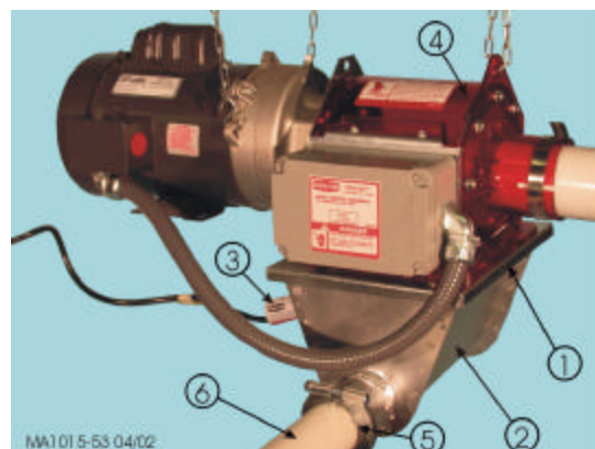
Figure 2. Fill System Control Unit/Terminal Boot Installation
